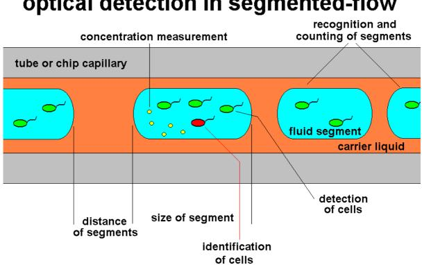
optical detection in segmented-flow
